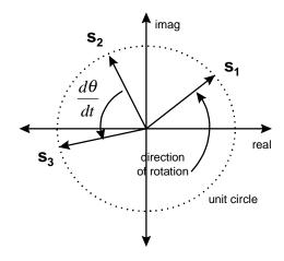
Figure 3.1-3 Rotating Phasor Representation of Transmitted Signal
