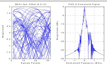
Figure 5.3-2 Composite PSD and Eye Diagram for 3 MHz Frequency Offset with Rx Filtering Removed
