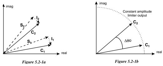
Figure 5.2-1 Case A: Interference at Same Frequency as Desired Signal
