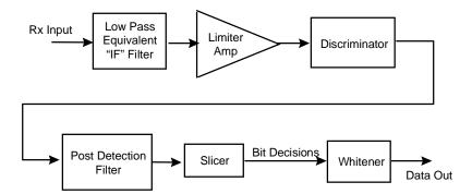
Figure 3.3-1 Baseband Limiter/Disriminator Receiver
