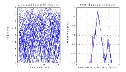
Figure 5.3-3 Composite PSD and Eye Diagram for 5 MHz (ACI) Frequency Offset with Rx
