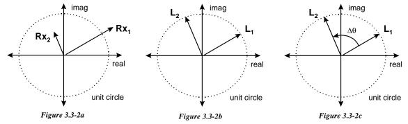
Figure 3.3-2 Vector Representation of Limiter/Discriminator Demodulation
