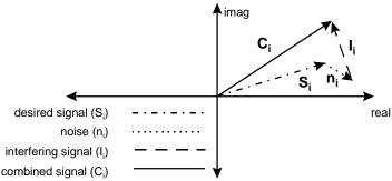
Figure 3.2-2 Linear Combination of Signal, Interference, and Noise
