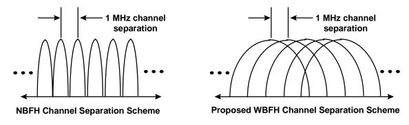
Figure 3.0-2 Channel Separation Schemes for NBFH and WBFH Systems
