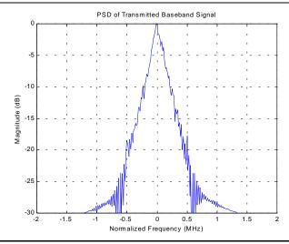
Figure 3.1-2 PSD of Transmitted 4FSK Signal
