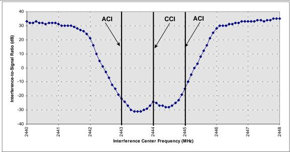
Figure 2.0-1 Rx Desensitization Data for 4FSK FHSS Radio (10<sup>-5</sup> BER Threshold)
