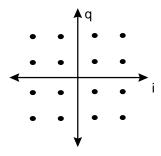
Figure 6.3-1 Signal Constellation for 16 QAM
