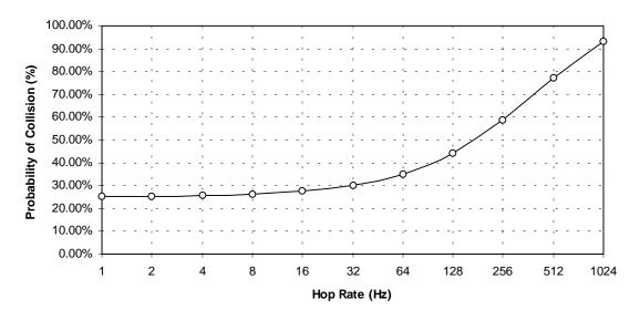
Figure 3.0-3 DSSS Probability of Collision as a Function of FHSS Hop Rate (1000 byte DSSS Packets)
