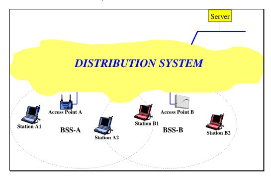
Figure 1 - Wireless LAN System Architecture
