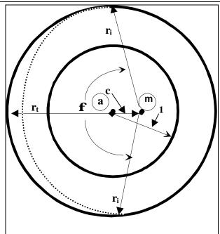
Figure 3-2. Configuration for Analyzing the Relative Number of WBFH Interferers.
