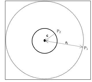
Figure 3-1. Illustration of the Interference Range Compared to the Communication Range
