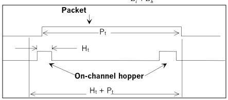
Figure 2-1. Illustration of WBFH Overlap with LAN Packet.
