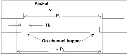
Figure 2-1. Illustration of WBFH Overlap with LAN Packet.
