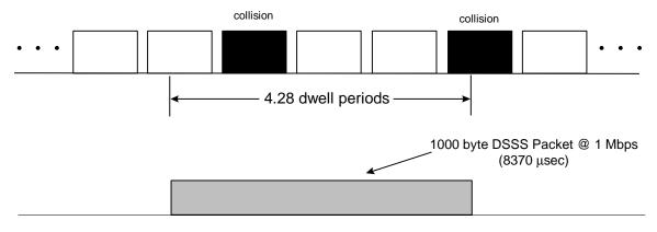
Figure 3.0-2 Increasing Hop Rate Increases Probability of Collision (FHSS System @ 512 hops/sec)
