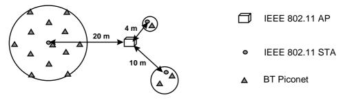
Figure 3.1.1-1 Number of Potential BT Interferors Depends on Range from AP
