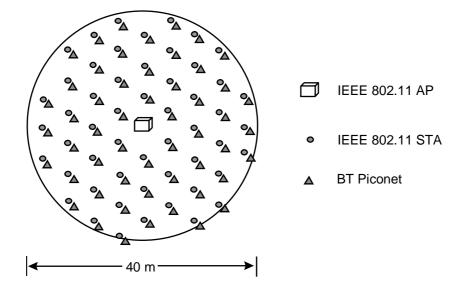
Figure 2.2.1 Composite BT/DSSS Network Topology
