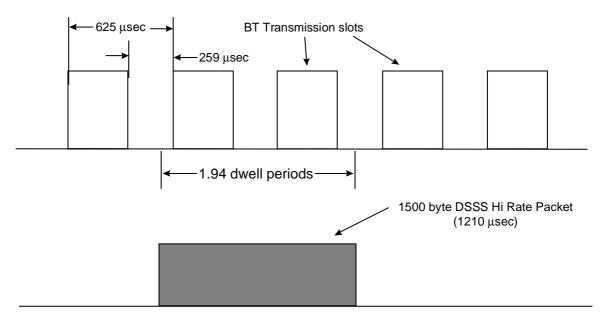
Figure 3.2.1-1 Probability of Collision Depends on Number of BT Slots Overlapped
