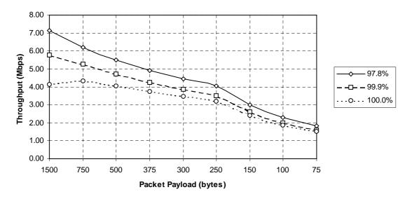
Figure 5.0-5Availability Curve for IEEE802.11WLAN in Presence of BT Interference(Range to AP = 4 m)
