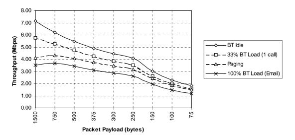
Figure 3.2.1-2 Throughput for DSSS WLAN as a Function of Piconet Utilization (Single BT Interferor)
