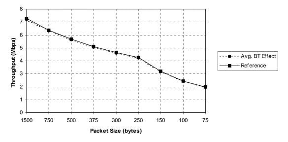
Figure 4.3-1 Average Effect of BT Interference Over an 8 - Hour Day
