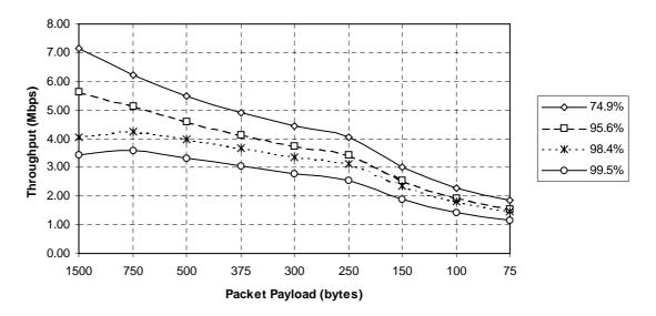
Figure 5.0-3 Availability Curve for IEEE802.11 WLAN in Presence of BT Interference (Range to AP = 20 m)
