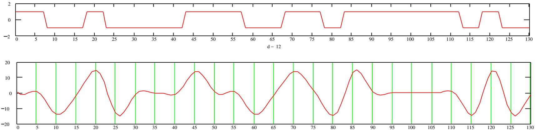
Shown below is a simulation binary data pattern and the resulting video waveform. At sampling time, the amplitude is either +1 or -1 for data 1 or approximately zero (several dB) lower for data zero.
