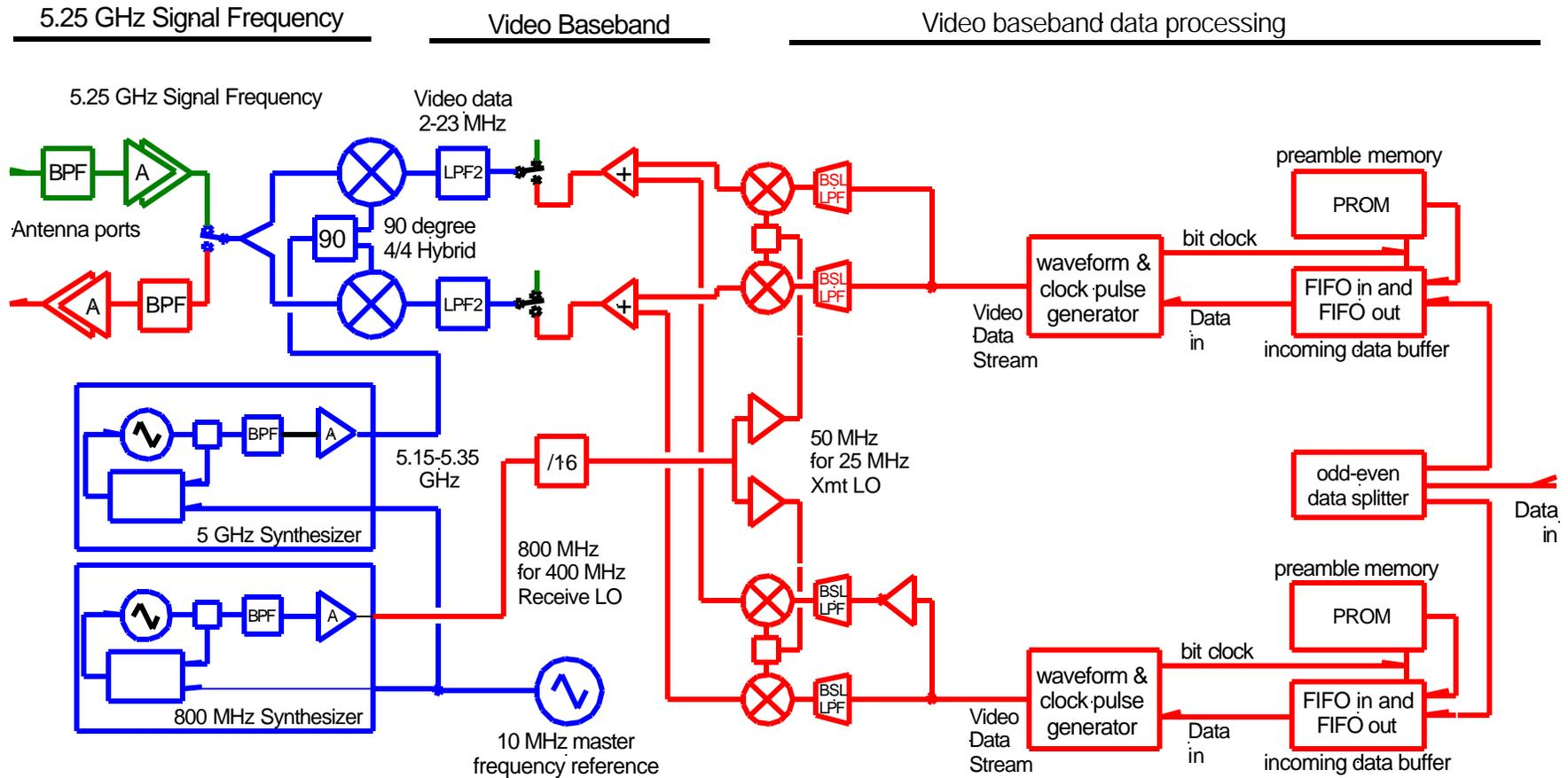
**Figure A-2 5.25 GHz dual ISSB AM data radio transmitter block diagram (60 Mbps in 48 MHz bandwidth)**
