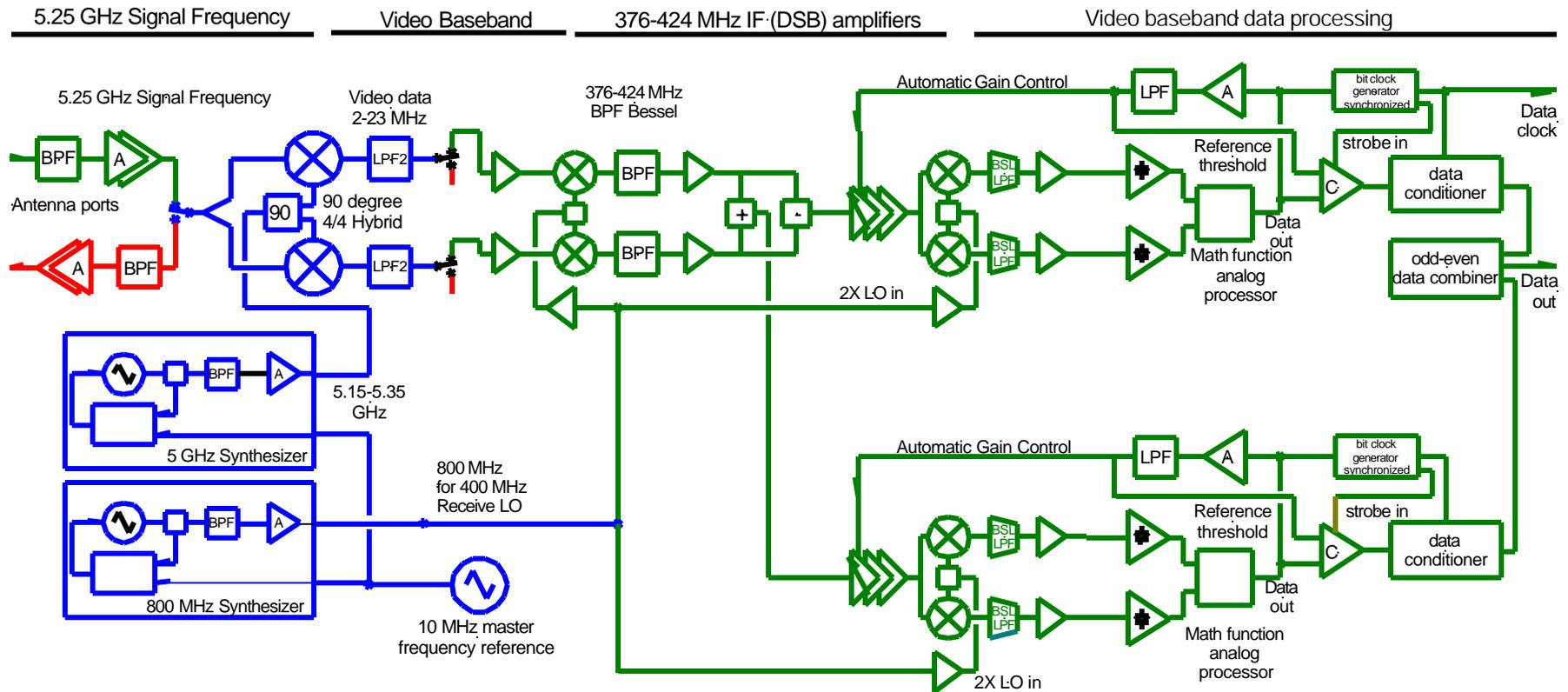
Figure A-3 5.25 GHz dual ISSB AM radio receiver block diagram
