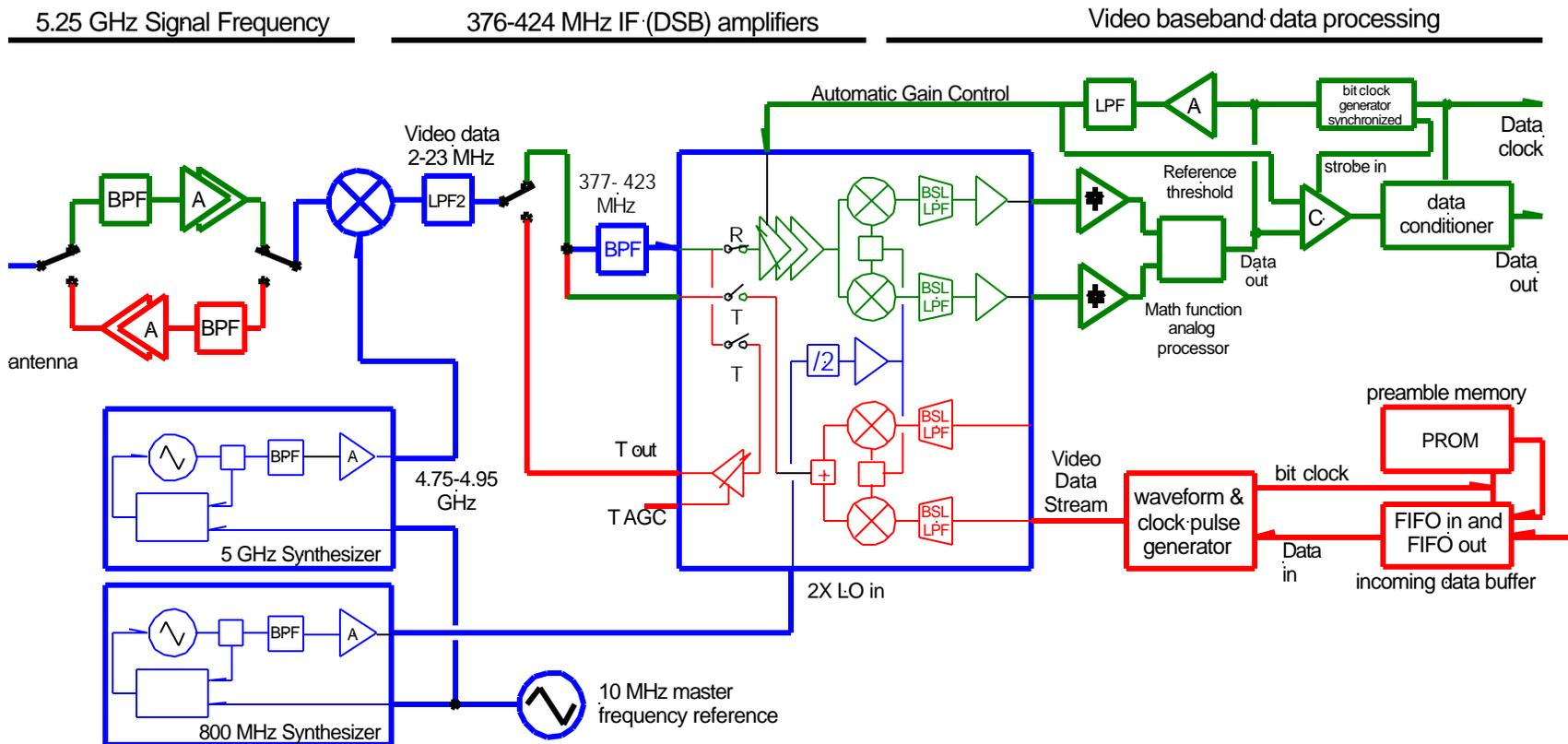
Figure B-1 AM DSBSC Radio Modem Transceiver Block Diagram
