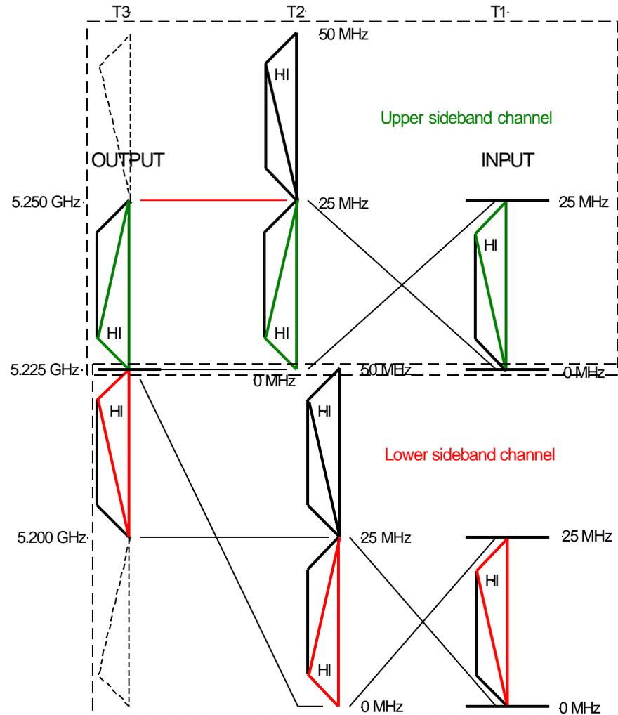
**Figure A-1 Frequency relationship diagram for transmit conversion steps**
