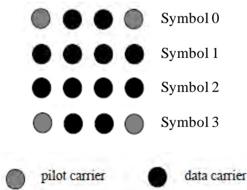
**Figure 332a—Description of a DL tile in VHF Mode**
