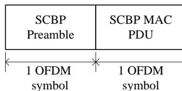
Figure 812—SCBP burst structure of WirelessMAN HR-OFDMA network.
