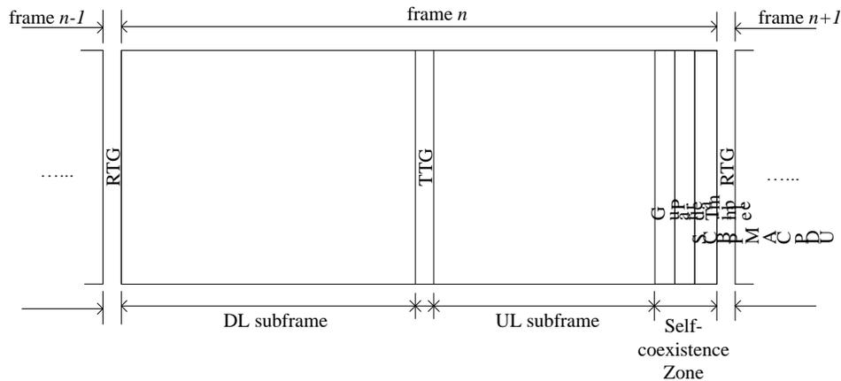
Figure 811—TDD frame structure with self-coexistence zone.
