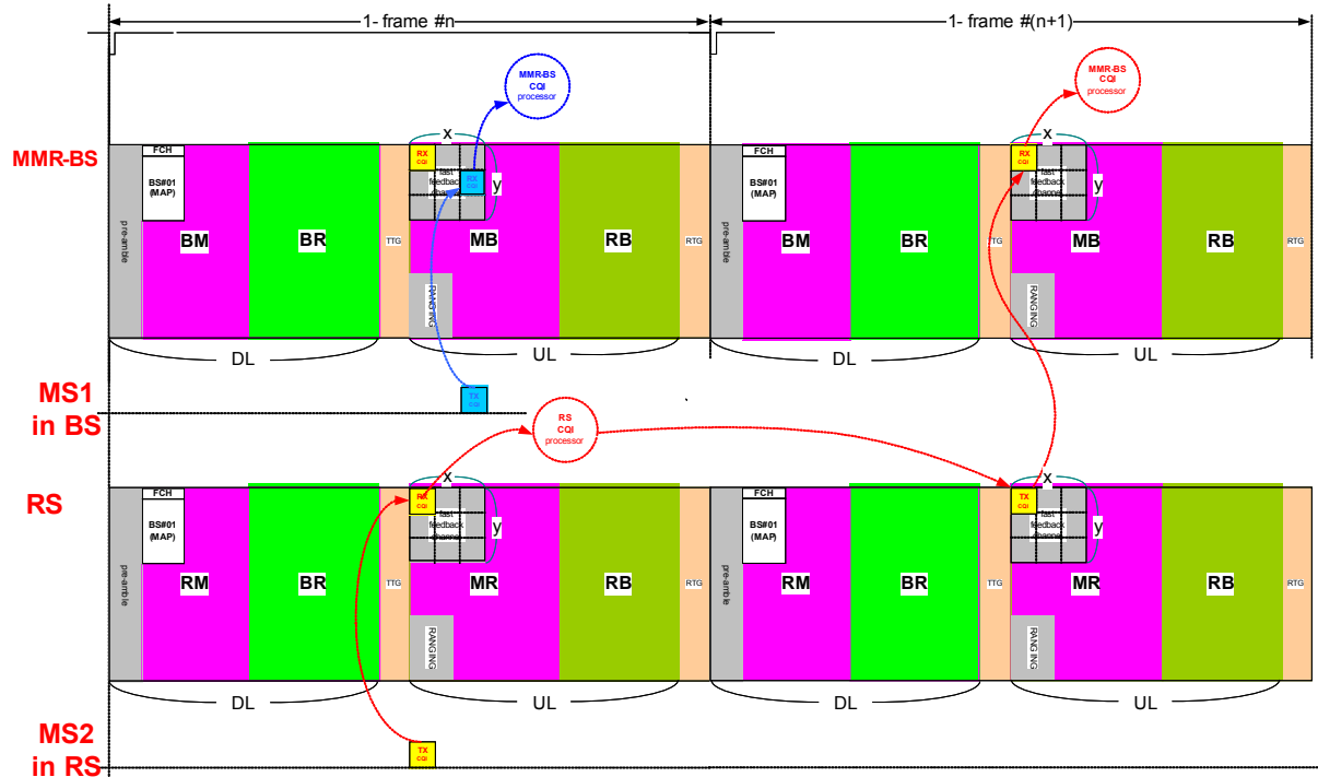
Figure 4. The example of fast feedback channel allocation in the case of using only one fast feedback channel region
