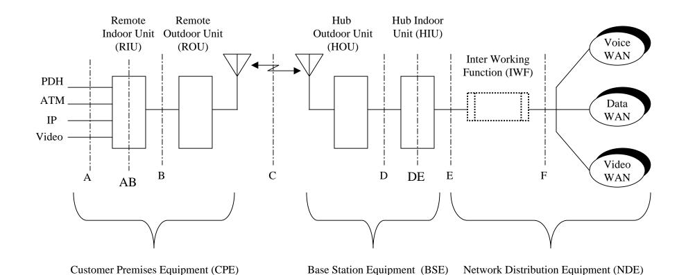
System Reference Point, which are described in the text, are labeled A-F
