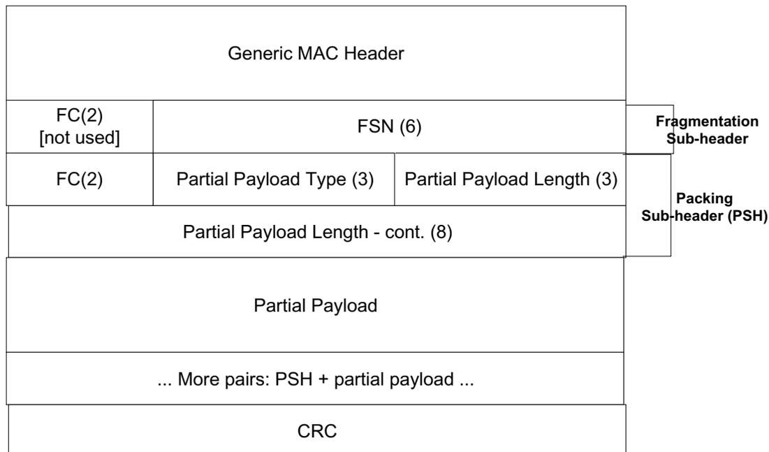
The invocation of the ARQ includes the definition of ARQ feedback (ACK, NACK) format(s). The packing functionality may be used for piggybacking ARQ related information (as well as another types of MAC signaling in the future) onto the data messages transmitted over the 802.16 wireless connection. So an indication needed for the type of partial payload that appears in the packed MAC PDU..
