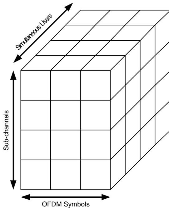
**Figure 1: Illustration of OFDMA2 PHY Burst Allocation**
