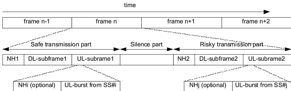
Figure 1 Proposed frame structure in the LE bands
