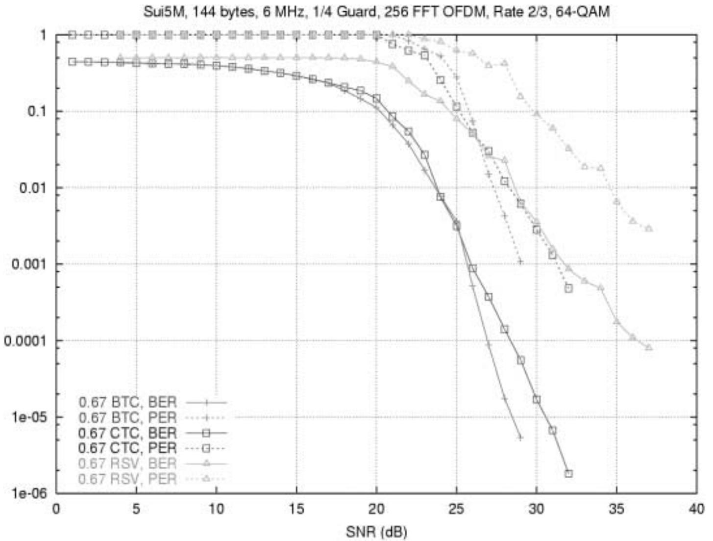
Figure 3 – Rate 2/3, 64-QAM on Sui5M
