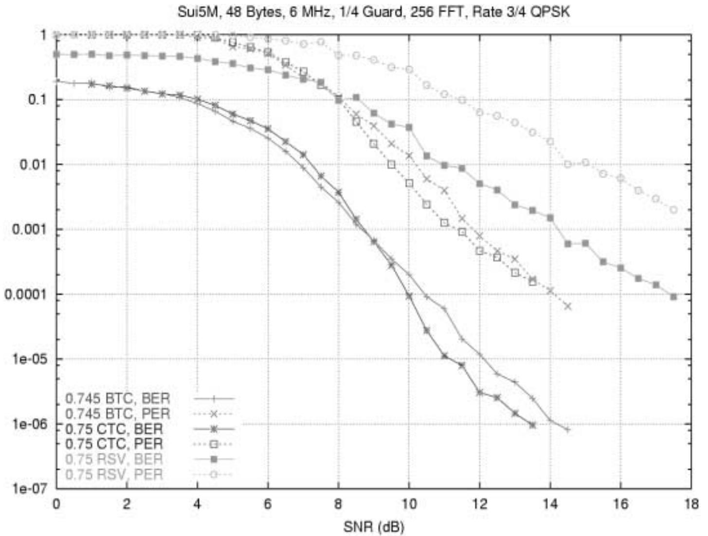
Figure 1 – Rate ¾ QPSK on Sui5M
