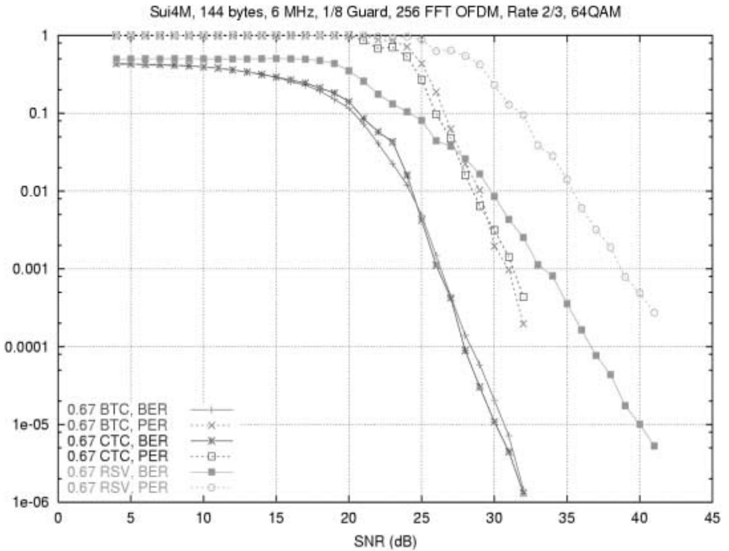
Figure 2 – Rate 2/3, 64 QAM on Sui4M
