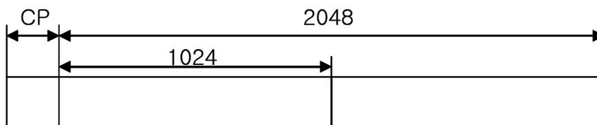
Figure 1-Time domain illustration of the DL preamble.
