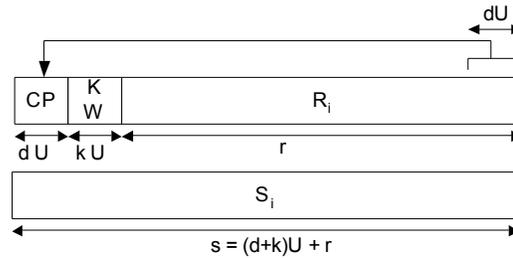
Figure 195—Formation of subchannel frame from frame segments
