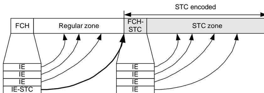
Such implementation eliminates the need to transmit the whole DL-MAP at BPSK that would increase the overhead.
