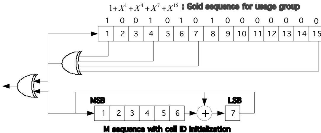
Figure 3 – PRBS for ranging code generation
