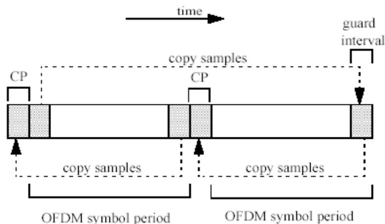
Figure 1 – Initial and HO ranging transmission for OFDMA
