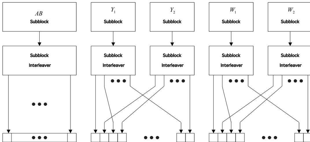
**Figure ccc— Block diagram of the interleaving scheme**
