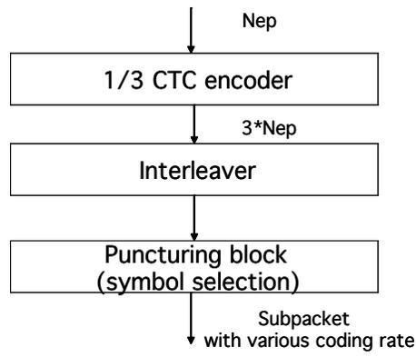
**Figure bbb— Block diagram of subpacket generation**
