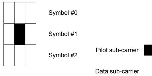
The allocated frequency band shall be divided into 552 tiles, the allocation of tiles to subchannels is performed in the following manner:
