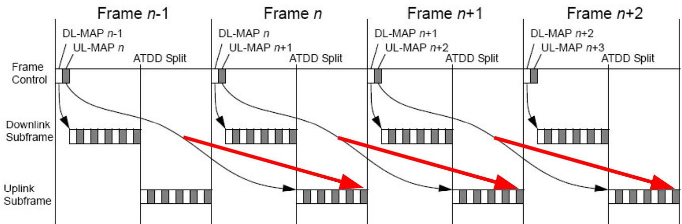
**Figure 44—Maximum time relevance of DL-MAP and UL-MAP(TDD)**
