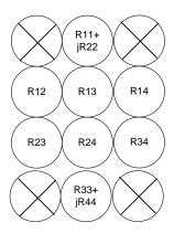
In this example we repeat the same mapping 6 times over all the tiles in one CQICH slot to provide diversity and interference immunity.
