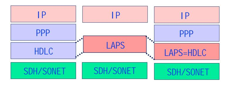
PPP over SDH/SONET IP over SDH
