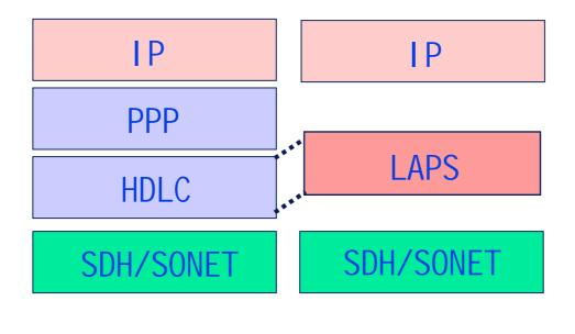
PPP over SDH/SONET IP over SDH
