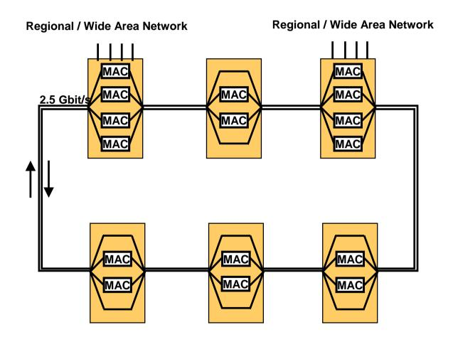
2.5 Gbit/s dual ring with electronic bypass nodes
