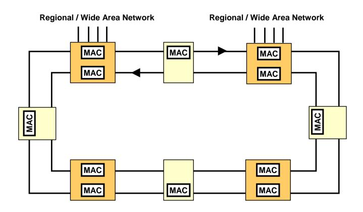
Collection / distribution ring with two gateway nodes and two high-performance nodes
