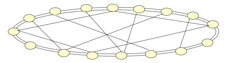
All links are wavelength channels on ring-structured fiber installation
