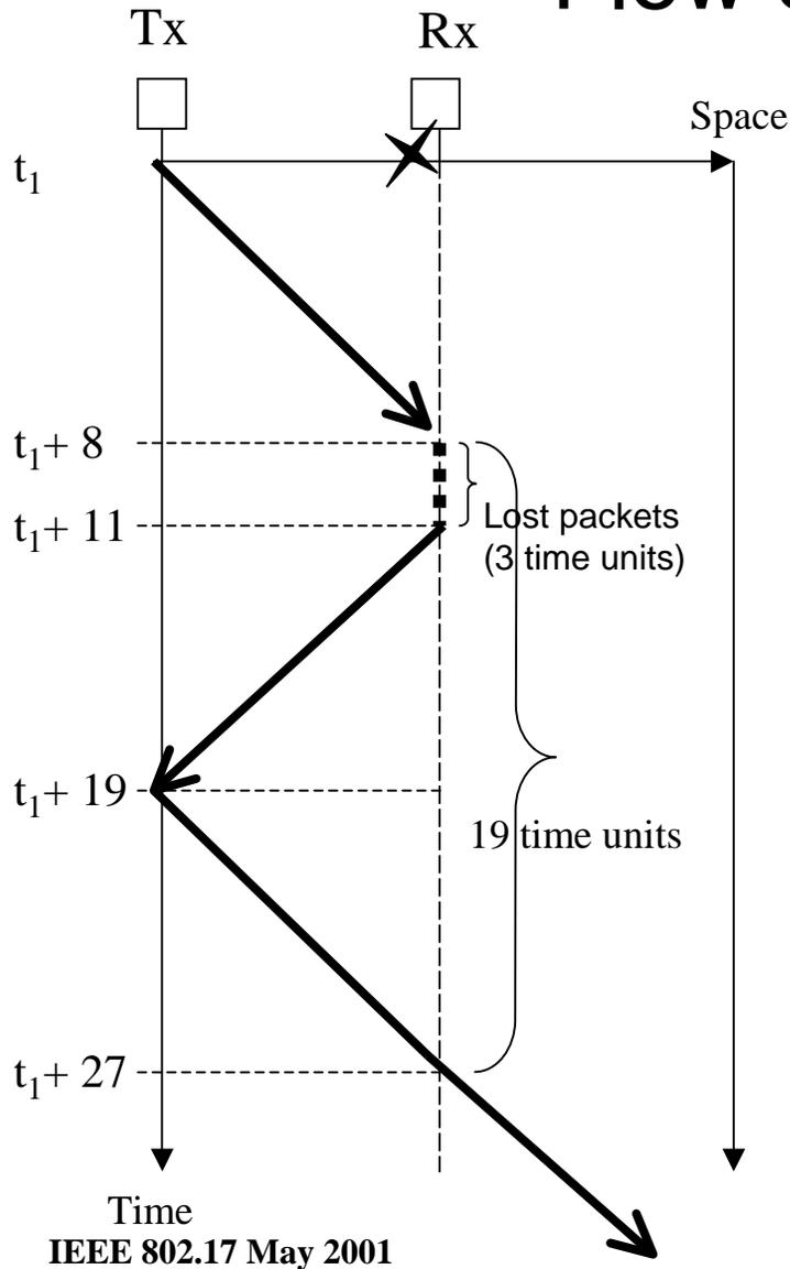
Ring delay between Tx node and Rx node (both sides) = 8
