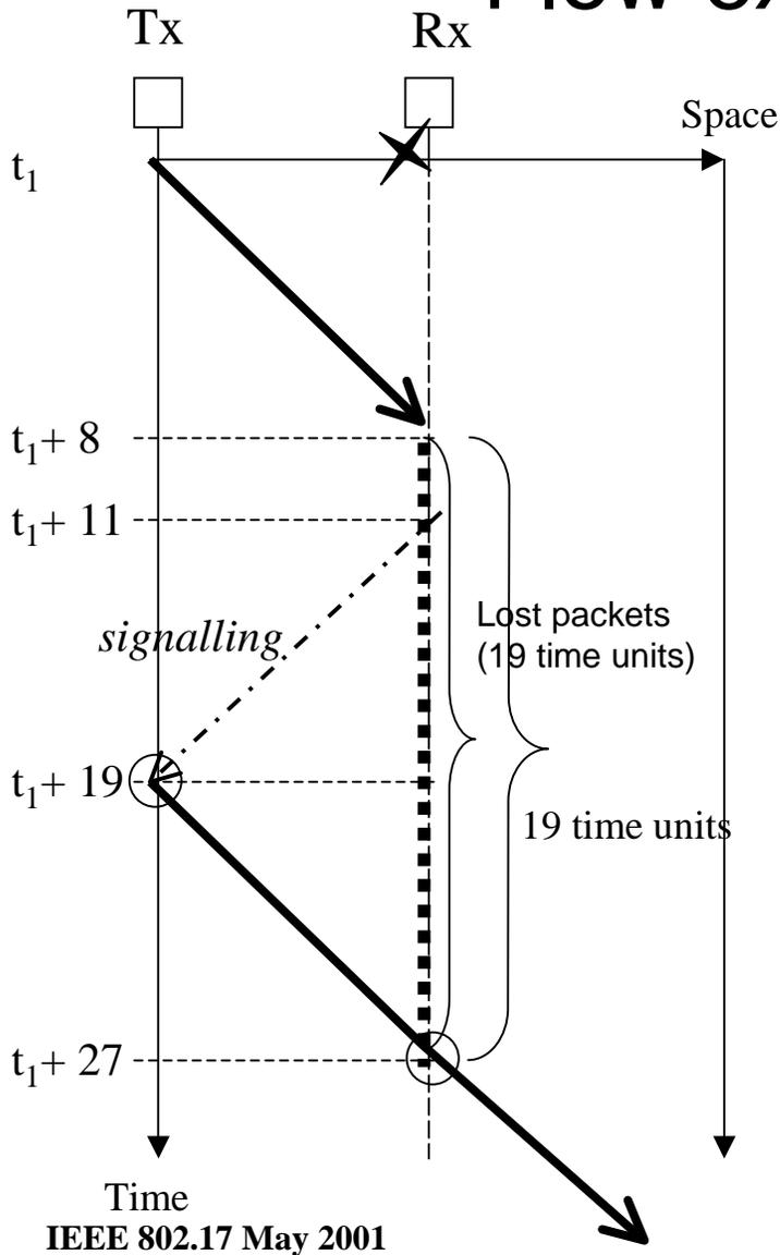
Ring delay between Tx node and Rx node (both sides) = 8
