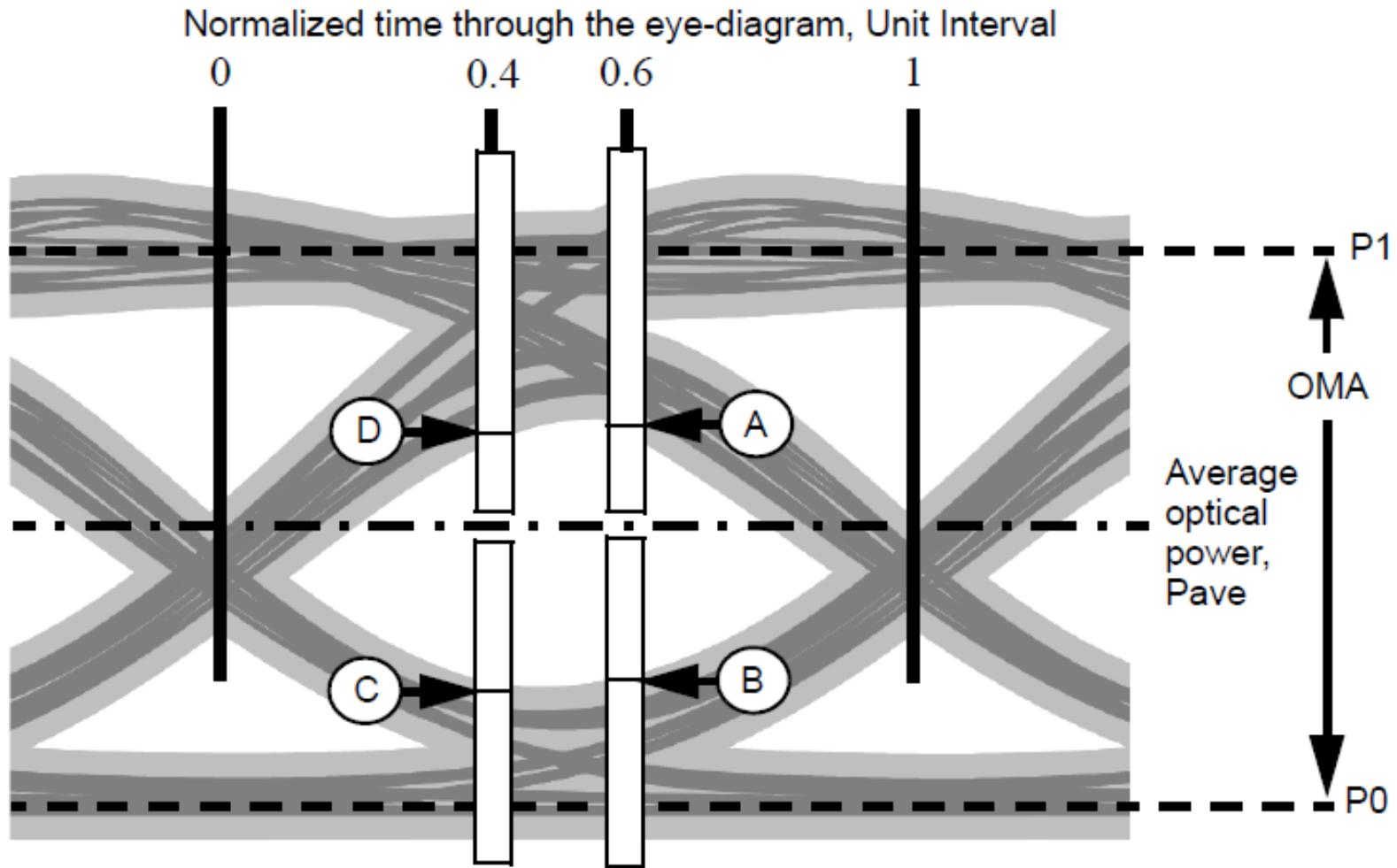
Figure 95–4—Illustration of the TxVEC measurement
