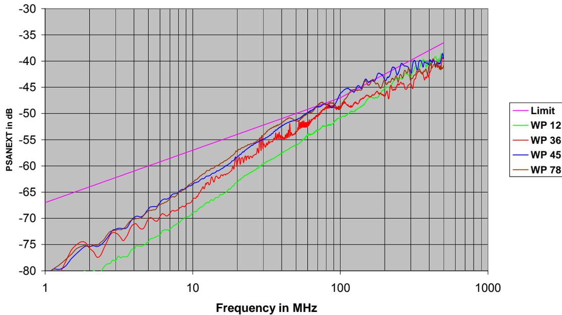
Figure 4: PSANEXT of victim channel 12 to all 47 disturber channels.
