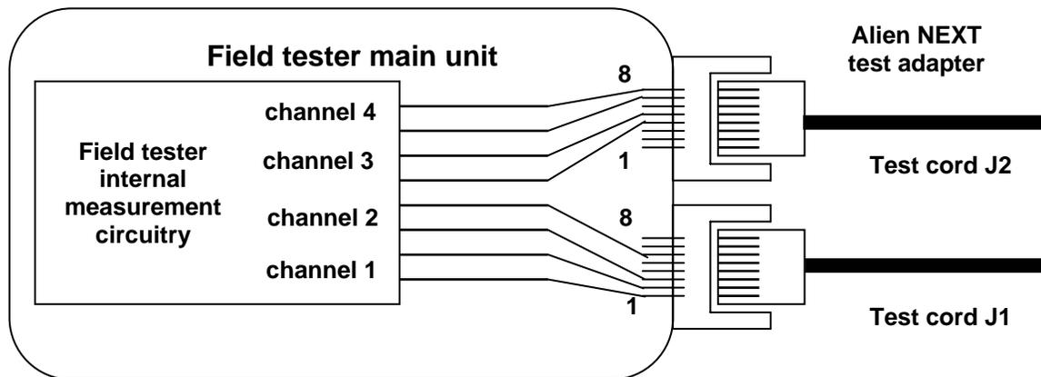
**Figure 1: Principle of use of a regular field tester for Alien Crosstalk measurements.**
