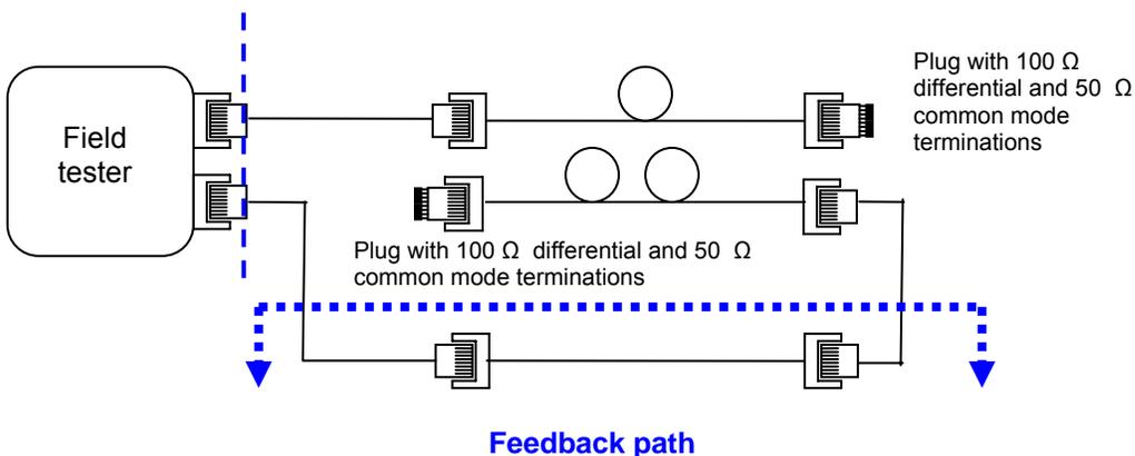
**Figure 2: Schematic diagram for the Alien FEXT measurement.**
