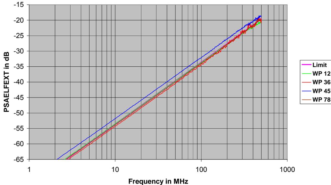
**Figure 6: PSAELFEXT of victim channel 12 to all 47 disturber channels.**
