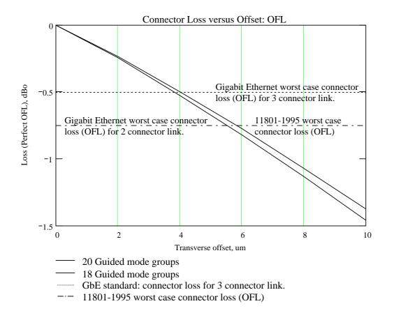
The loss graph was calculated using overlap integrals between the modes of nominal 62.5/125 multimode fibre.
