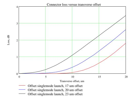
• The loss graphs were calculated using overlap integrals between the modes of nominal 62.5/125 multimode fibre. Connectors are assumed to be physical contact therefore no reflection loss.
