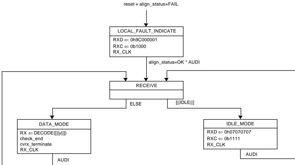
Figure 48-9—PCS receive state diagram
