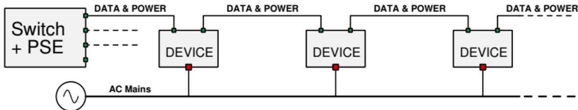
Devices (luminaires, sensors, ...) are connected in passive linear topology. DALI carries a limited amount of power, and offers bus based data at very low data rate.
