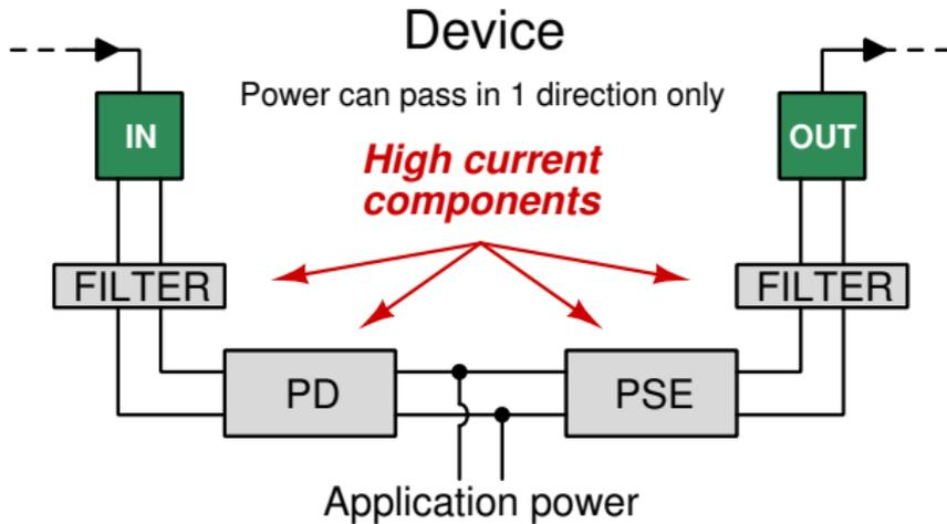
If the device must block DC power, then a PD+PSE construction is needed, or at the very least in and output filtering. All of these components must be rated for the full output current of the source PSE, which is orders of magnitude larger than the current requirement of the application in the device. Power flow is unidirectional.
