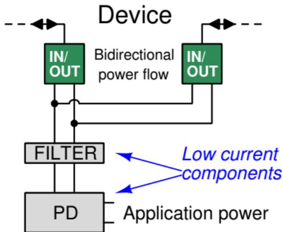
If at DC frequency it is possible to directly connect the “in” to the “out” connector, there is no cost associated with transferring power through the device. The PD components only need to be rated for the device’s own power consumption. Power flow is bidirectional.
