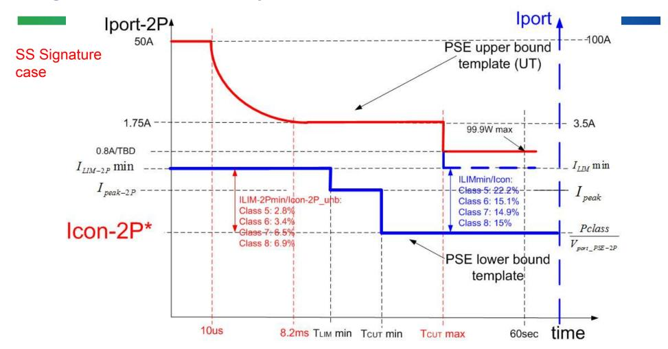
(\*) Icon-2P can vary between Icon – I1 to Icon-2P unb were I1 it the other pair current. Icon-2P is equal to Icon-2P unb at the worst case. The total current that PSE has to support is Icon and not 2xIcon-2P\_unb. The actual current on the pair set may be lower according to the following equation: Icon-2P=min (Icon – I1, Icon-2P unb).
