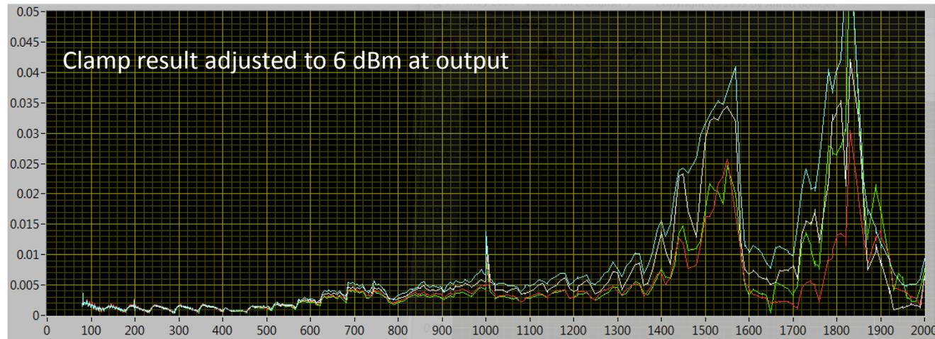
Result adjusted as if 6 dBm is maintained at the clamp output
