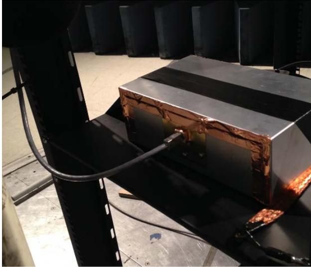
A termination box and channel were mounted in a representative NEBS test configuration
