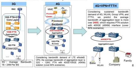
**Extended reach(>10km)** interface is essential for inter-building connections without long-haul transmission systems.
