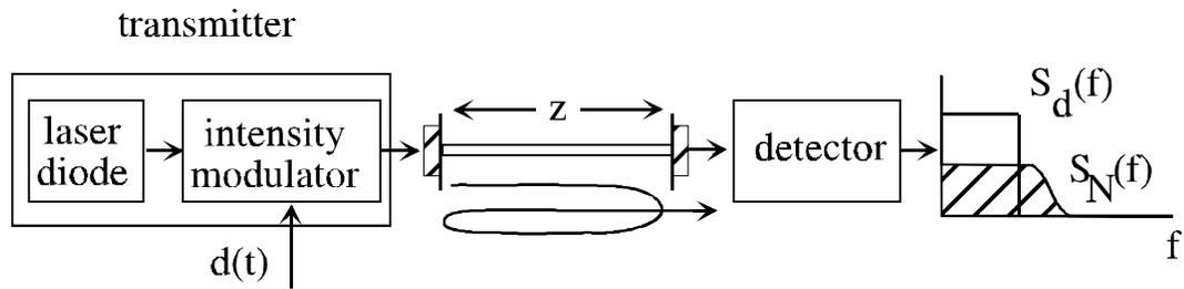
**FIGURE 1.** Fiber-optic link experiencing multiple reflections from fiber interfaces (connectors, fiber ends etc.). The graph right of the detector shows schematically the data spectrum  $S_d(f)$  accompanied with the interferometric noise, whose power spectral density is  $S_N(f)$ .
