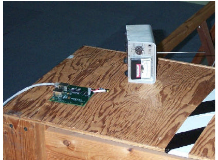
DTE Load Board with LED load below the minimum load
