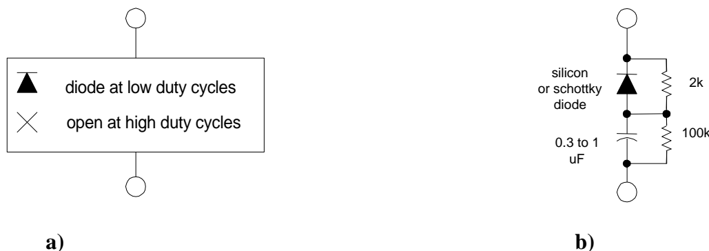
Figure 5, proposed PD identity network: a) block diagram form, b) schematic form
