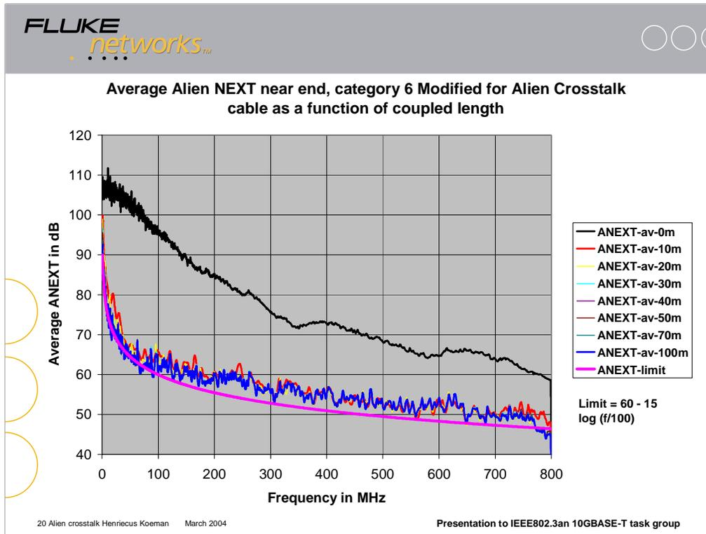
This slide shows the average Alien NEXT, as measured from the near (=taped together) end as a function of taped length.
