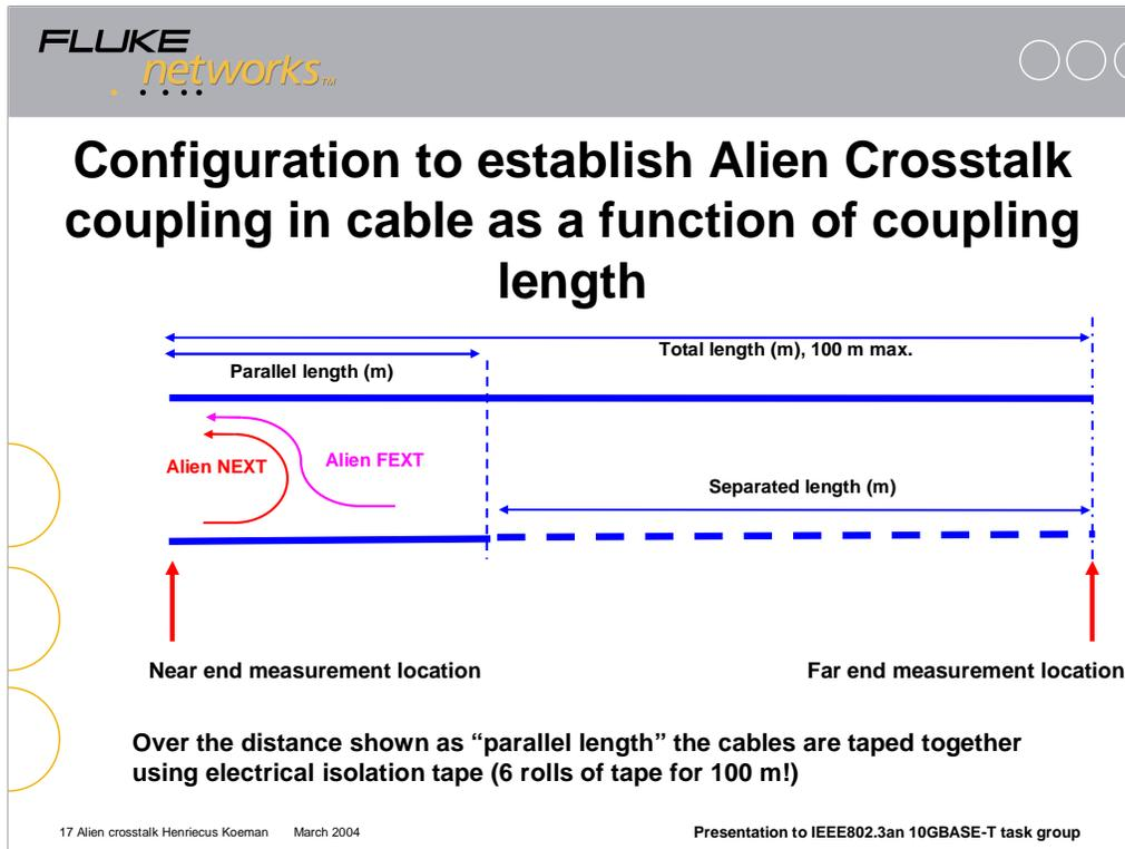
This slide shows the test configuration of the Category 6 cables with enhanced Alien Crosstalk performance to determine the properties as a function of joint by taping length. This experiment was NOT conducted on the Category 5e rated cable.
