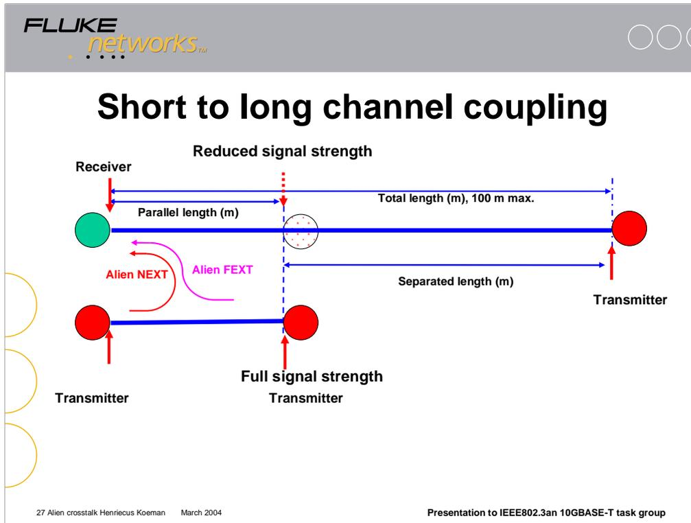
This slide shows the potential trouble from (EL)FEXT coupling when a short channel runs in parallel with a long channel.
