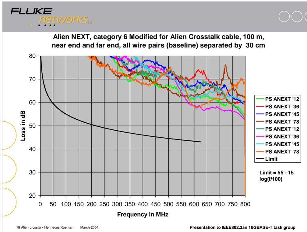
This slide indicates the measurement floor. In this test conditions, the two cables were separated over the full 100 m length by between 30 cm and 50 cm.
