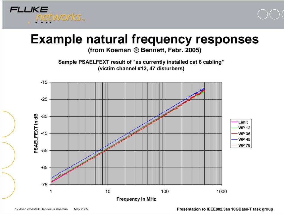
Alien ELFEXT is extremely well behaved and closely approaches a 20 dB/decade slope. Therefore very likely a fail condition at low frequencies will cause a fail condition at high frequencies as well.
