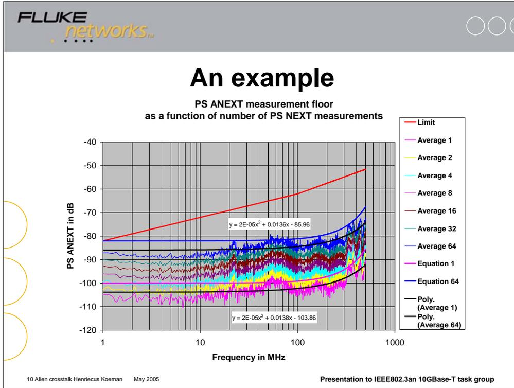
This slide shows the degradation of a random noise floor as a function of the number of measurements that is included in a PSAXtalk result. With the number of cables that may be in a cable bundle (48) in one example, one can observe that the limits at low frequencies can easily reach into the expected random noise floor.
