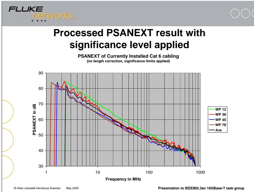
This is the data that remains after post-processing using the “significance” level approach.
