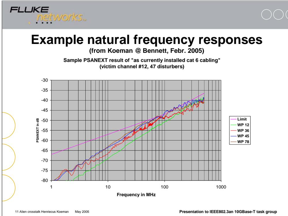
We claim that we really should not worry too much about passing limits at low frequencies. Both alien NEXT and alien (EL)FEXT exhibit behavior that is well predictable, we can therefore assuming with high confidence that a failure at high frequencies will cause the same at low frequencies and vice versa.
