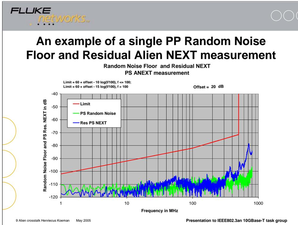
This slide shows an example of a random noise floor and residual AXtalk for a PP ANEXT measurement. The random noise floor is almost -110 dB over the 1 MHz to 100 MHz range and then declines to approx. -100 dB at 500 MHz. Given that there is a trade-off between measurement time (IFBW) and noise floor, this is about as good as what one can practically obtain.
