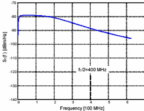
$$Mask(f_{MHz}) = \begin{cases} -78 \text{ dBm/Hz}, & 1 \leq f \leq 330 \\ -78 - \left(\frac{f-330}{40}\right) \text{ dBm/Hz}, & 330 < f \leq 1850 \\ -116 \text{ dBm/Hz}, & 1850 < f \leq 3000 \end{cases}$$
