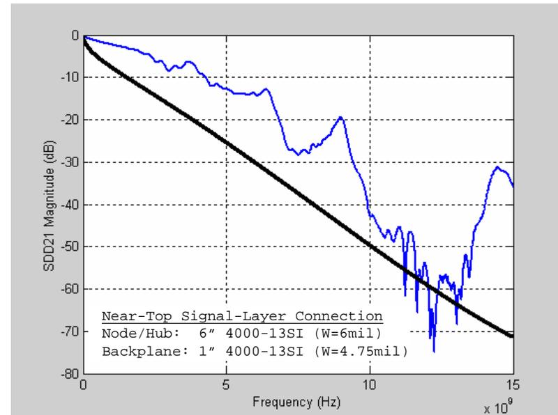
**Current mask fails channels with significant stub-related resonances.**
