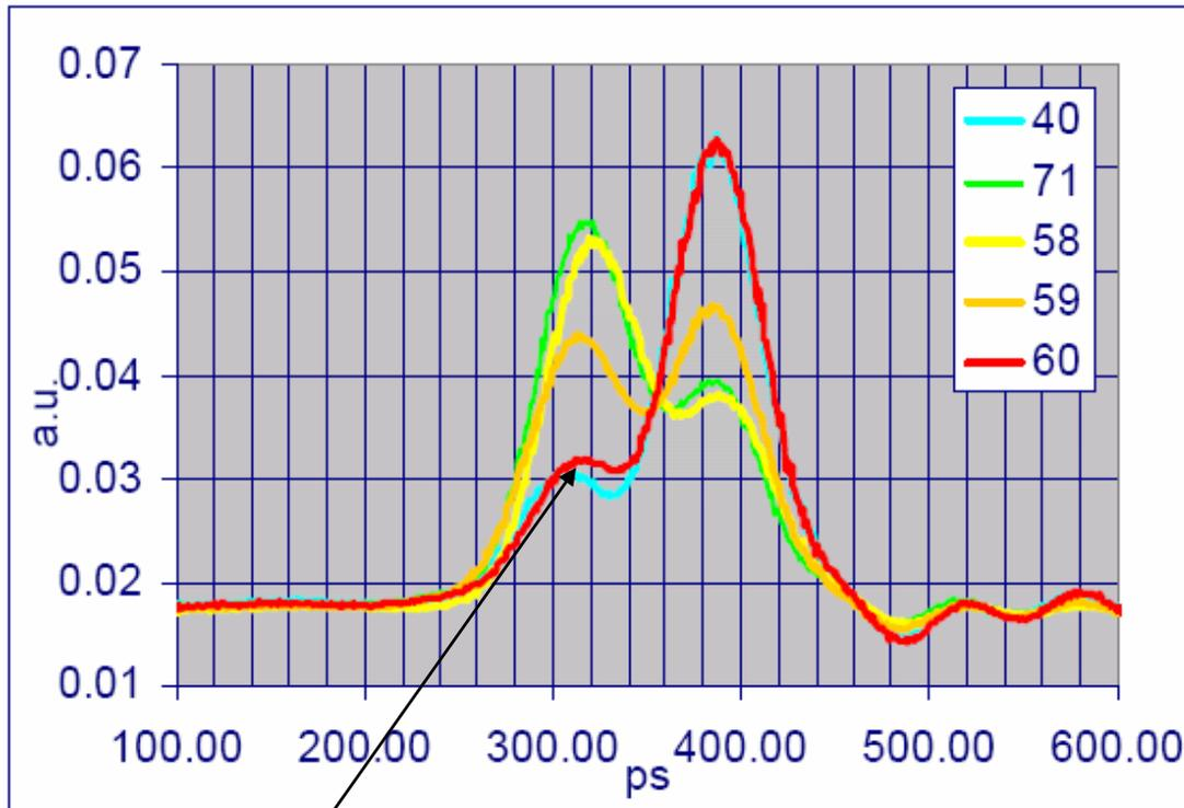
**Corning experience is that we don't see the "infinite bandwidth" with 0um-1um launch with fibers with pulse splitting which is noticeable with 4um offset.**
