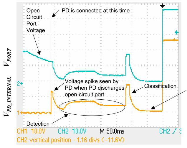
In this example, port goes to 0V which would reset the PD state machine. However, that is not required per IEEE 802.3af
