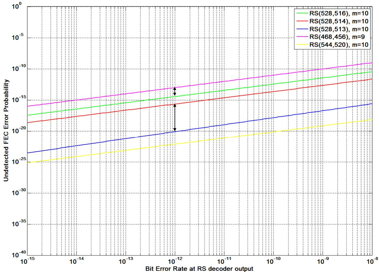
RS(528,513) has 28,100x less undetected FEC errors than RS(528,514) at target BER=1e-12.
