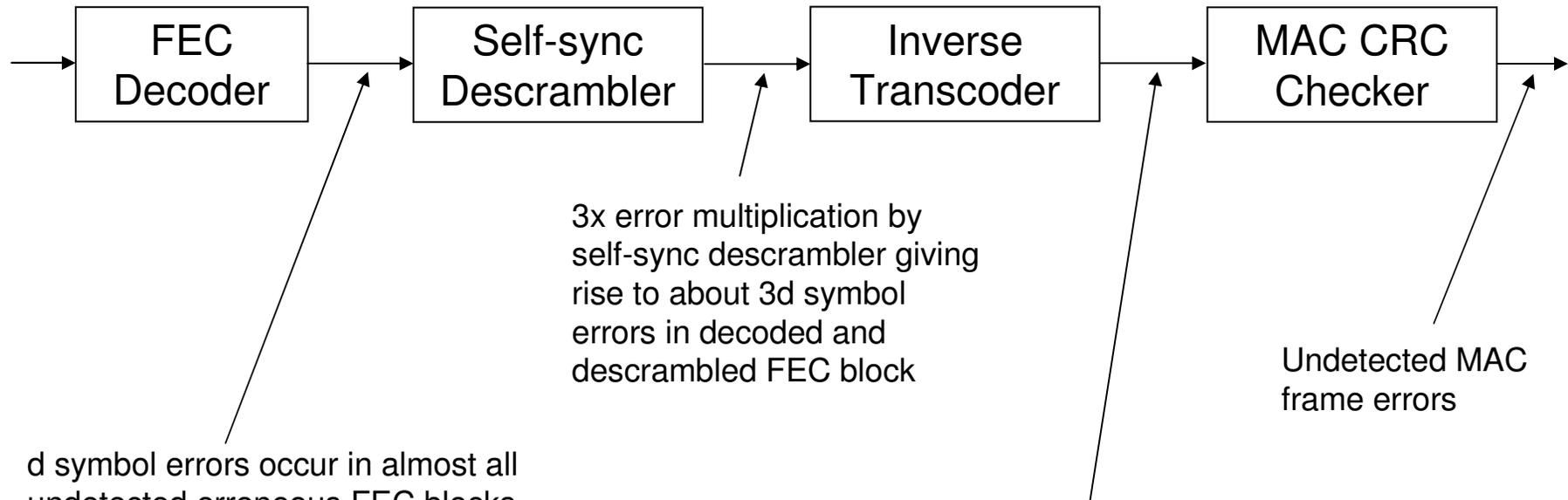
$d$  symbol errors occur in almost all undetected erroneous FEC blocks where  $d = n - k + 1$  is the minimum distance of the  $RS(n,k,t,m)$  code
