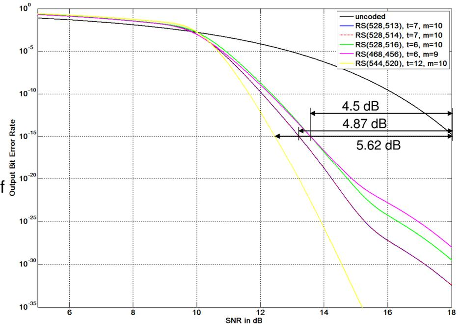
*Probability that next bit in a burst at DFE output is in error is b=0.5 for all computations in this presentation*
