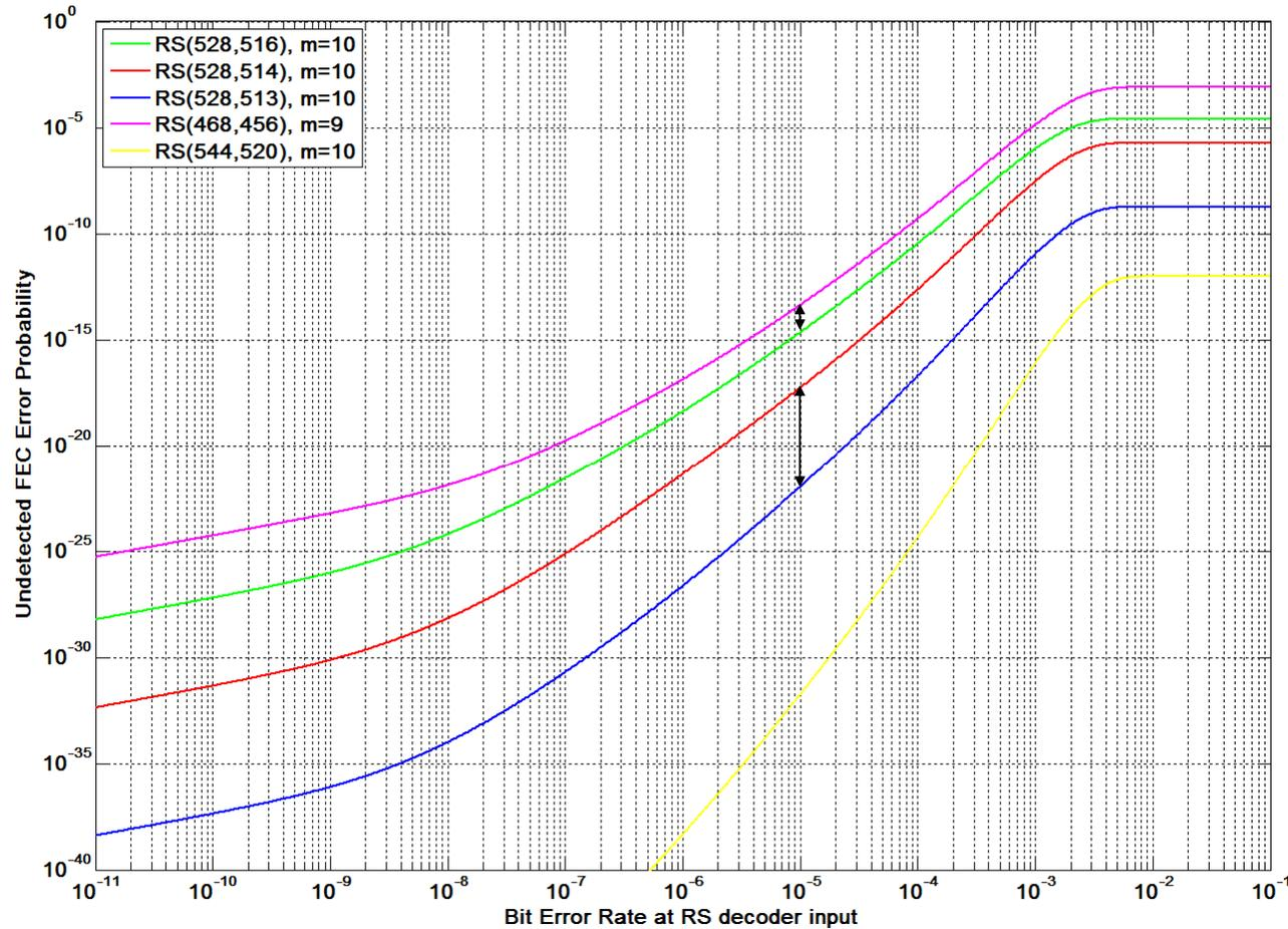
RS(528,513) has 100,000x less undetected FEC errors than RS(528,514) at DFE BER= $1e-5$ .
