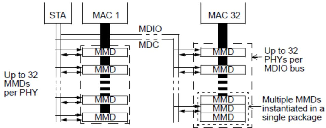
Figure 45-1—DTE and MMD devices
