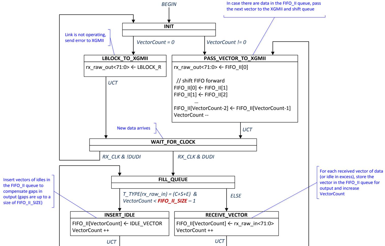
The same state diagram (see above) can be reused with proper changes of FIFO\_II\_SIZE:
