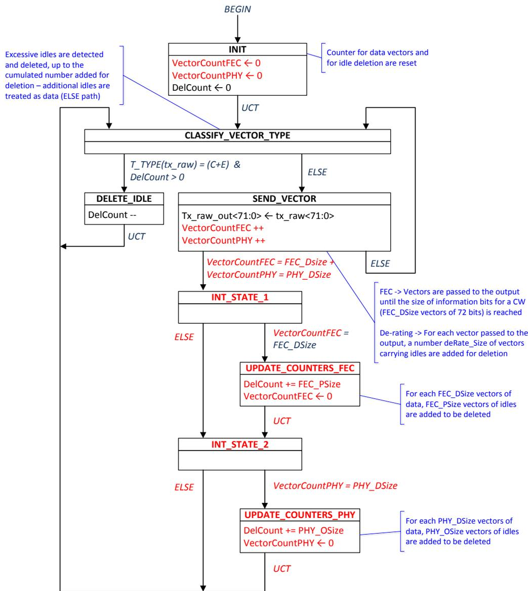
In **red** the change due to de-rating from the original chart – final format and proper rounding can be defined once know PHY parameters
