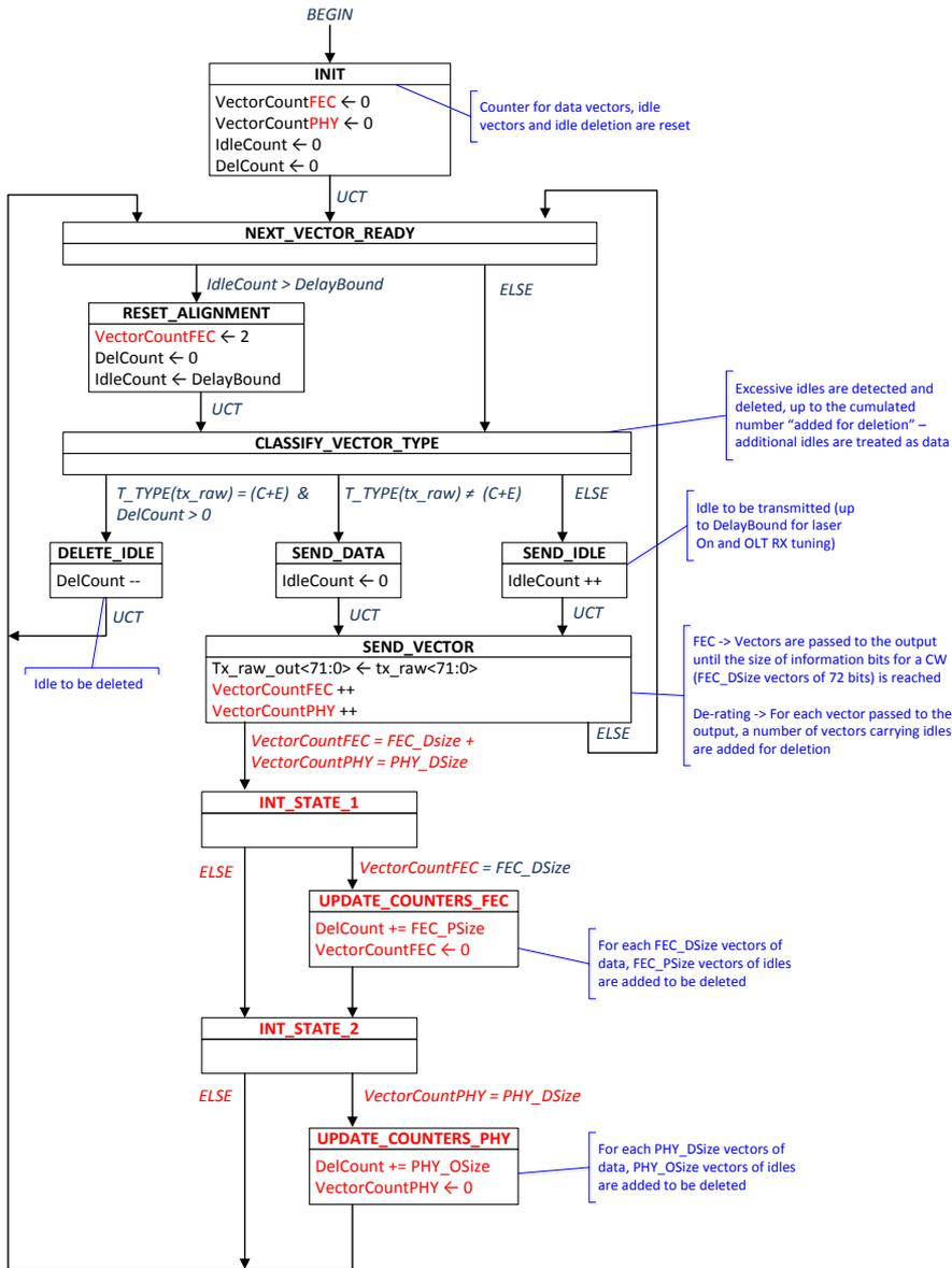
In **red** the change due to de-rating from the original chart – final format and proper rounding can be defined once know PHY parameters
