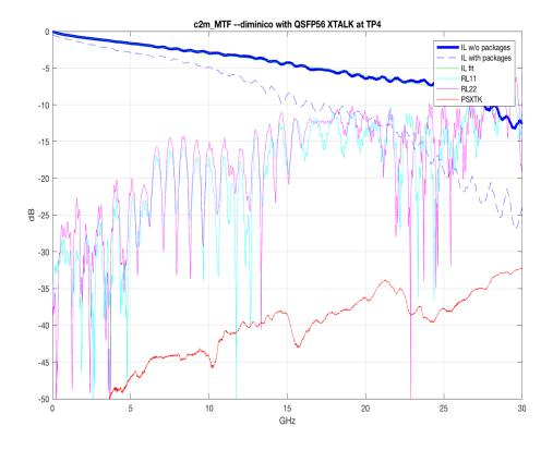
Results for std transmitter with A\_fe=0.9, A\_ne=1.26: VEO\*=67.7 mV (failing), ICN=2.9 mV, Peak ISI=24.1 mV, MDFEXT Peak=12.2 mV, MDNEXT=2.95, ILD(FOM)=0.055, COM=5.8 dB TP5: VEO=31.2 mV
