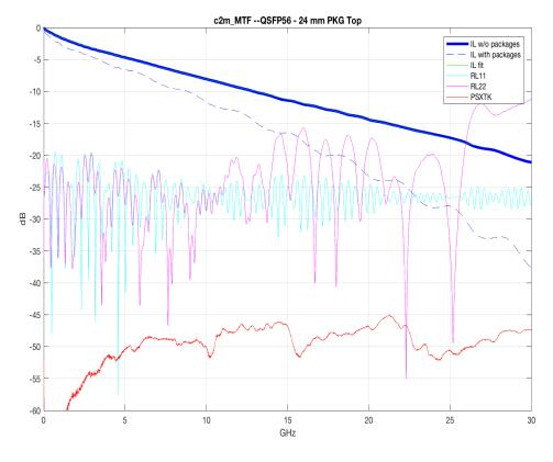
Results with Std TX: VEO\*=26.8 mV (failing), ICN=1.435 mV, Peak ISI=9.77 mV, MDFEXT Peak=2.6 mV, MDNEXT=0.51, ILD(FOM)=0.042, COM=4.97 dB
