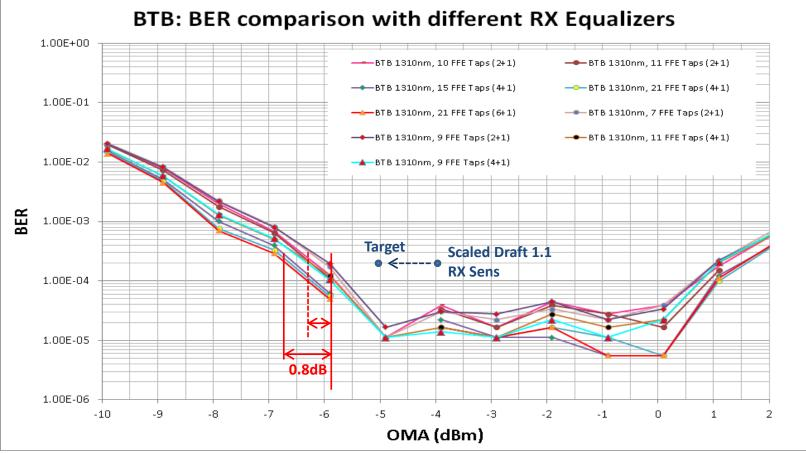
There's a good «flat» range between 0 to -5dBm range (@53G, -0.5 to -6dBm). Observed around 0.4dB penalty between 7 (2+1) and 9 (4+1) FFE (T/2) taps equalization. Other further 0.4dB improvement are achieved with more taps (15/21 T/2 spaced).
