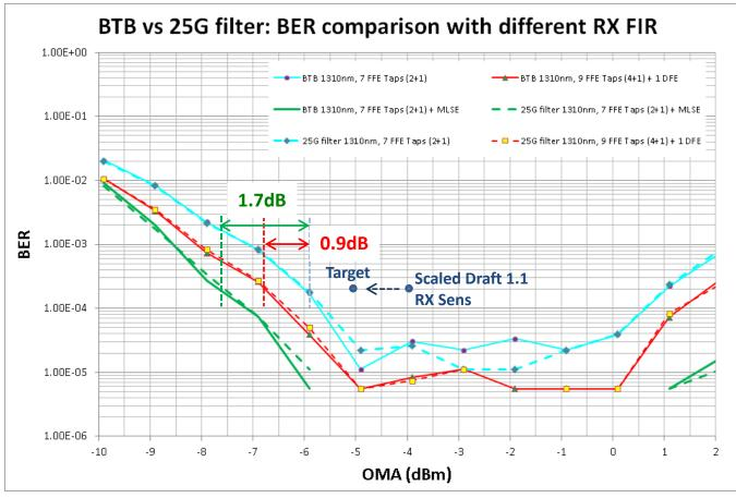
25GHz BW filter used, to simulate more restricted BW components.
