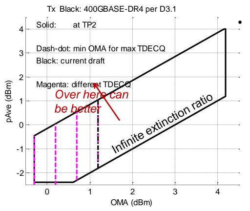
A single Tx waveform measurement is used to find TDECQ, OMA, mean power, and extinction ratio
