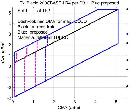
• A single Tx waveform measurement is used to find TDECQ, OMA, mean power, and extinction ratio
