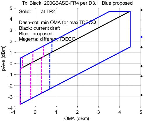
• A single Tx waveform measurement is used to find TDECQ, OMA, mean power, and extinction ratio Black polygon (partly hidden under blue one): Tx spec in D3.1, with 4.5 dB min. extinction ratio
