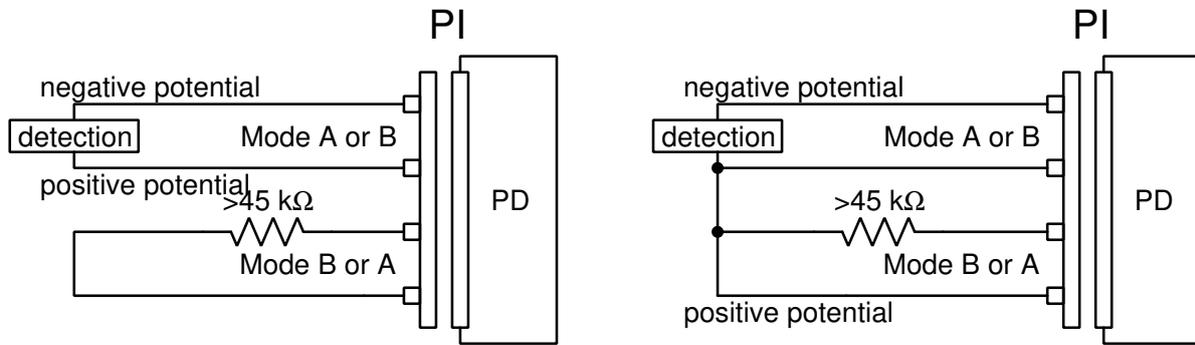
**Figure 145-27a — Detection signature requirements connection configurations**
